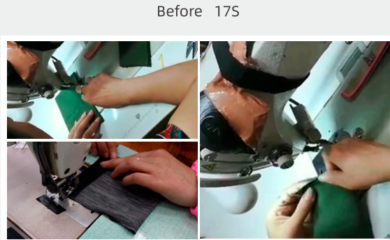
缝合 折翻 二道工序 Stitching, folding two operations
