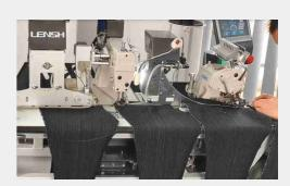
缝合压线一次完成 Stitching and pressing are completed at one time
